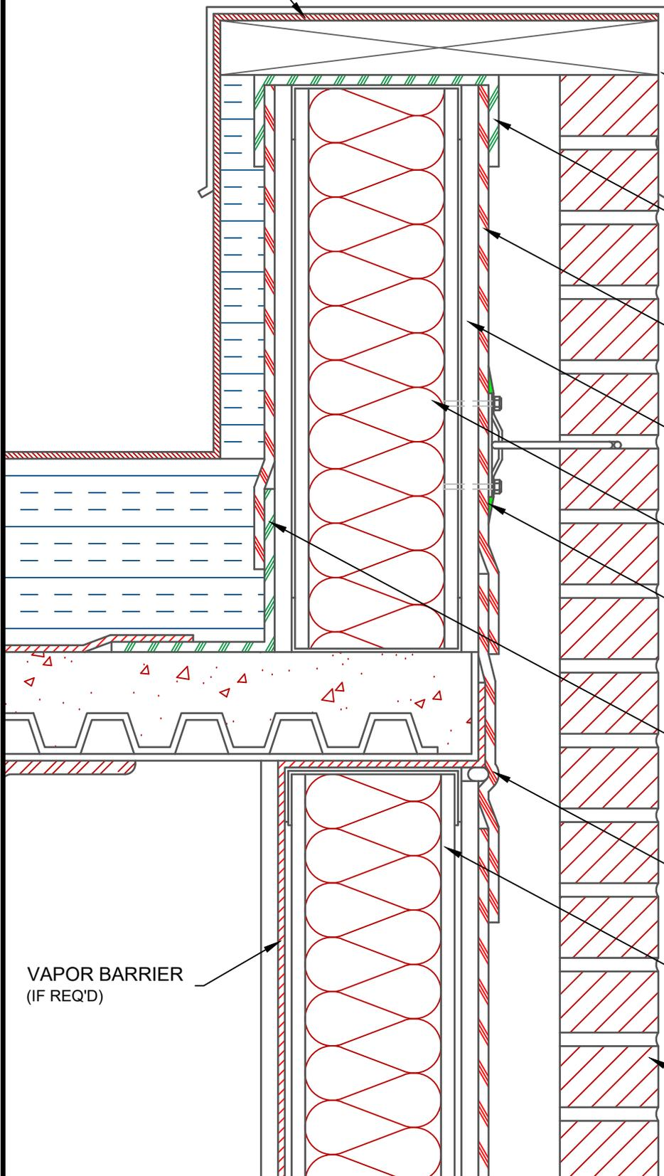
ROOF CAP FLASHING
